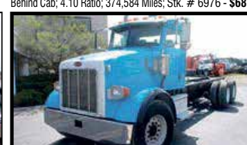
2005 PETERBILT 357 CAB & CHASSIS ; Cummins ISM 385 HP; Jake Brake; Allison Auto. Trans.; 20K F/A; 46K Rears; 252" WB; 21' Frame Behind Cab; 168" CT; Chalmers Susp.; Rear Engine PTO (REPTO); Frame Has Been Sandblasted and Painted; 68,882 Miles and 14,682 Hours; Stk. # 6924 - $56,900
